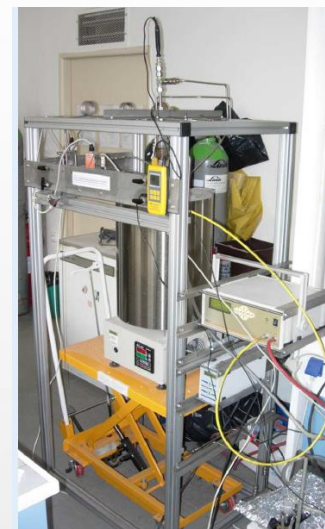
Experimental unit for high temperature CO 2 sorption (UCT)
