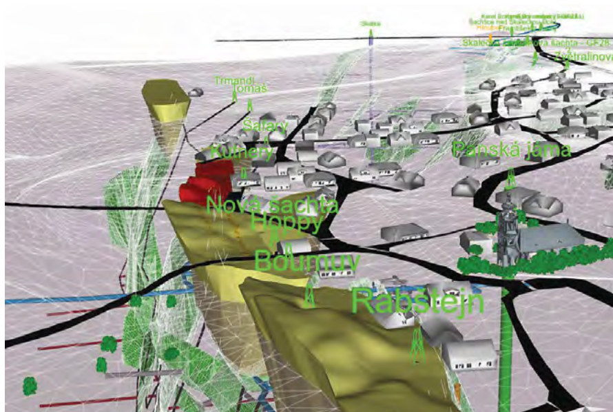
Comprehensive model of the Kaňk polymetallic ore deposit, featuring a 3D mineralization model, a Landscape model of development, a 3D model of mine workings, and a 3D model of undermining impacts. Author: J. Jelínek.
