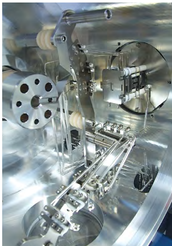
Chamber of the thermal ionization mass spectrometer (TIMS) with samples prepared for measurement. Photo by F. Laufek.
