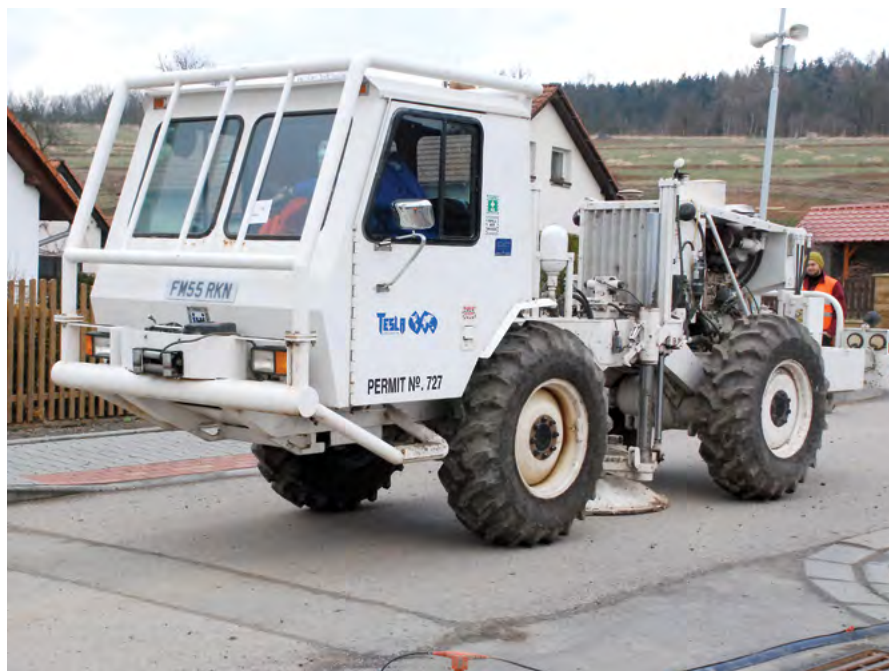
Vibroseis – seismic wave source, with a cable and geophone in the foreground.
