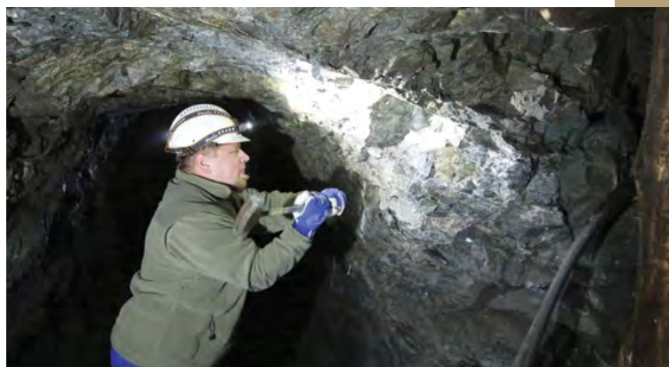
Bulk sampling of scheelite ore, Kristýna adit. Photo by V. Žáček.
