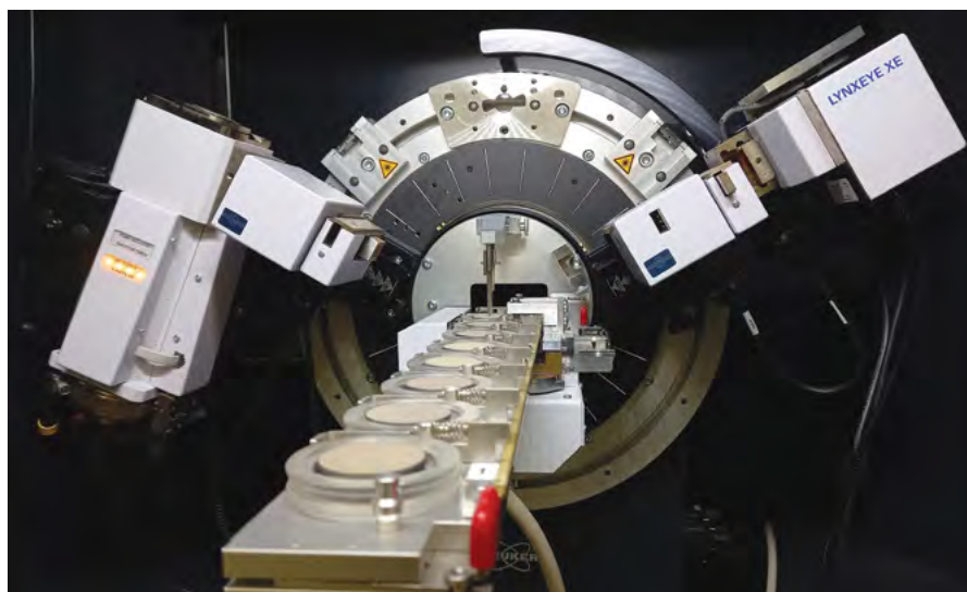
Goniometer of the Bruker D8 Advance X-ray diffractometer with an automatic sample changer. Photo by F. Laufek.
