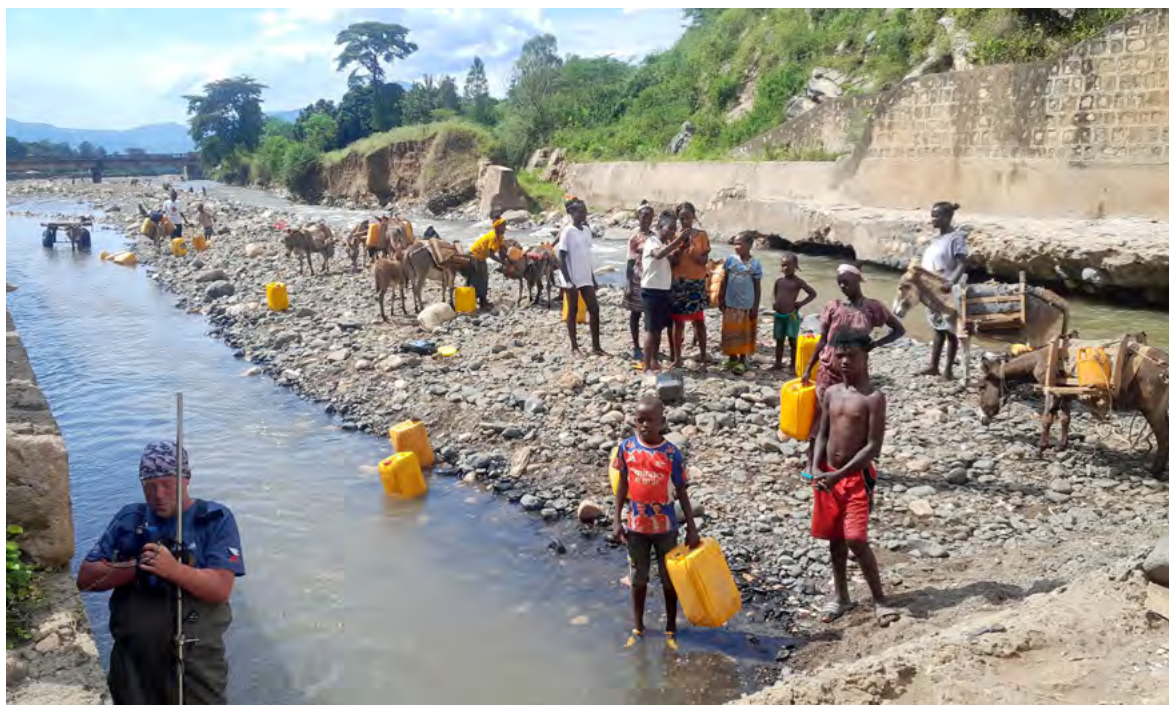
Measuring flows with a magnetic-inductive flowmeter on the Loma River in Ethiopia. Photo by J. Jelínek.
