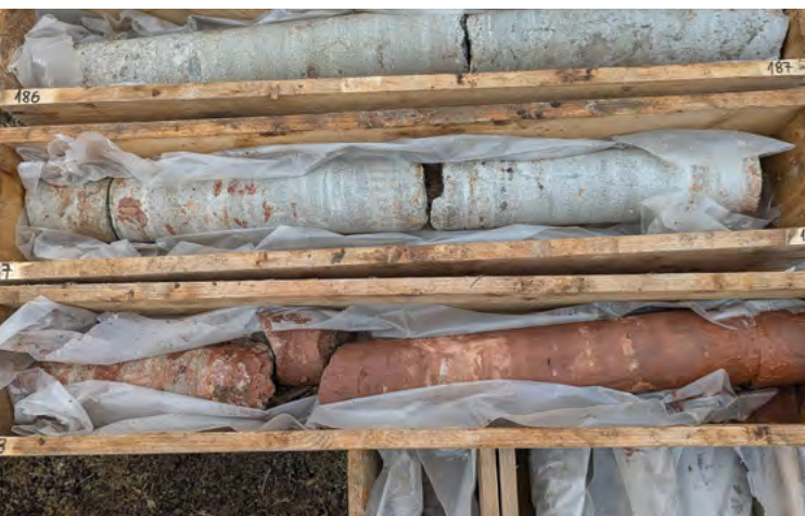
Drill core from the newly constructed 500-meter deep geological borehole at the Litoměřice locality. The section of the drill core from 186–189 meters shows the transition from light Cretaceous sediments to red Permian claystones. Photo by J. Holeček.
