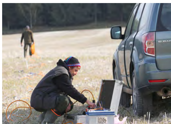
Field geophysical measurement using Electrical Resistivity Tomography (ERT) method. Photo by V. Žáček.
