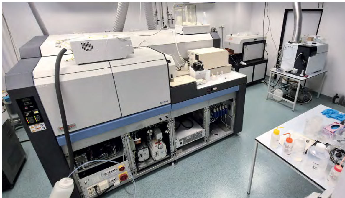
From left: multicollector inductively coupled plasma mass spectrometer (MC-ICP-MS), laser ablation (LA) system, and quadrupole inductively coupled plasma mass spectrometer (ICP-QMS). Photo by O. Šebek.
