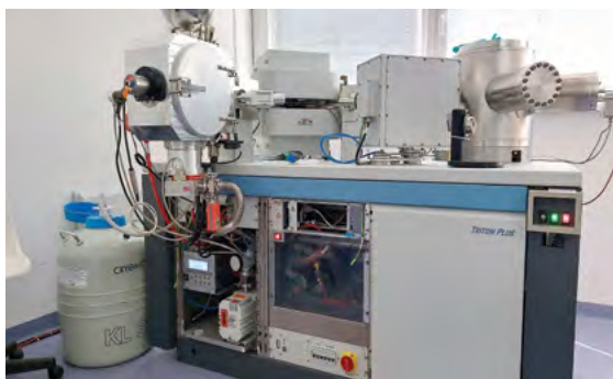
Laboratory of Mass Spectrometry uses the modern Triton Plus instrument for highly precise determinations of strontium and neodymium isotopic composition. Photo by T. Magna.
