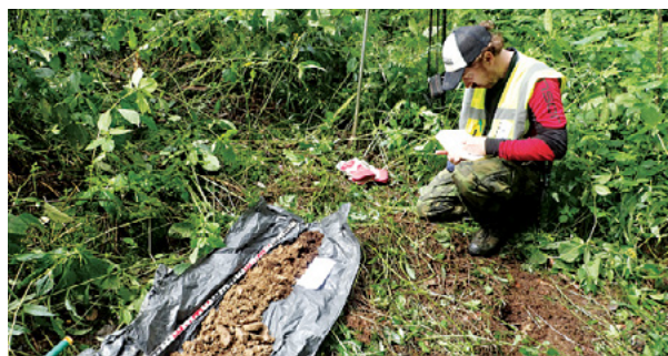
▲ Collecting metallometric samples from test pits at the Utín locality during the RENS project. Photo by P. Rambousek 2021.
