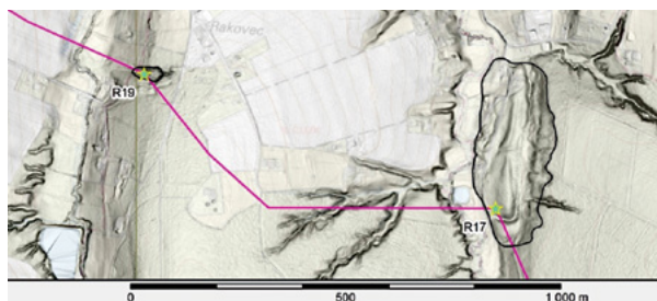
▲ Polygons (black lines) with occurring geodynamic phenomena were demarcated by geomorphological analysis of a 5 th generation digital terrain model (© ČÚZK). On the left, an erosional depression is evident with slopes affected by assumed slope movements (pylon R19), on the right, an area of a compound slope instability with a frontal shape (pylon R17).
