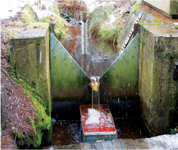
▲ Sharp-crested measuring weir in the Pluhův bor catchment (the brown water in the flow measurement vessel is due to a high concentration of organic carbon). Photo by P. Krám.
