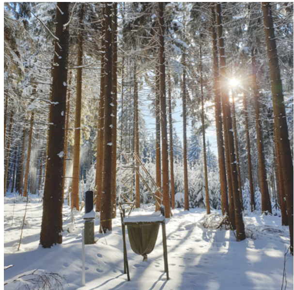
▲ Winter collector of atmospheric precipitation and litterfall trap for plant organs – Načetín, Krušné hory Mts. Photo by J. Čuřík.
