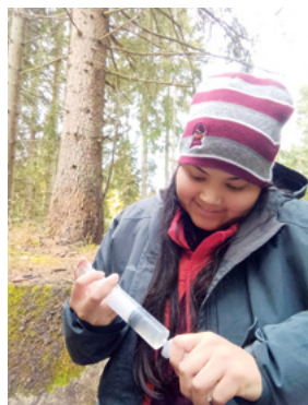
▲ Filtration of water in the Pluhův bor catchment for analysis of cations and trace elements. Photo by P. Krám.
