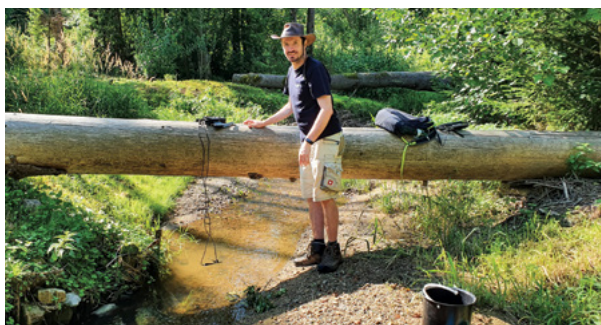
▲ Flow rate measurement of the Kyselá voda Stream near České Budějovice using the salt dilution method, PERUN project. Photo by J. Holeček.
