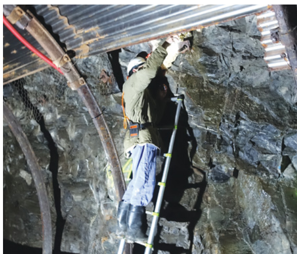
▲ Sampling of groundwater from a research borehole near the newly excavated underground research laboratory of the Radioactive Waste Repository Authority in the Rožná mine. Photo by L. Rukavičková.
