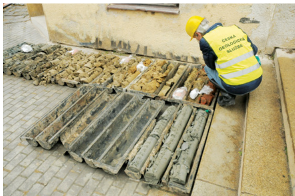
▲ Czech Geological Survey employees making a log of the engineering geology borehole on Anenská Street in Brno. Photo by O. Krejčí.
