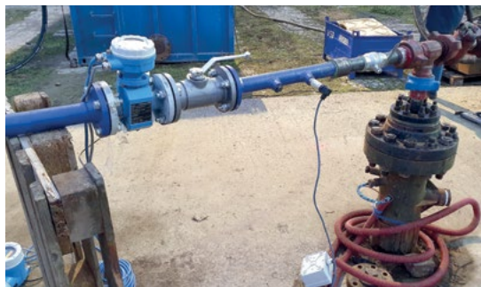
▲ Wellhead of the exploratory geothermal well PGV LT-1 in Litoměřice during hydraulic injection tests. Photo by J. Holeček.
