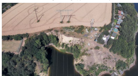
▼ A landslide area above the right bank of the Nechranice reservoir threatens a high voltage pylon. Photo by Martin Dostalík.
