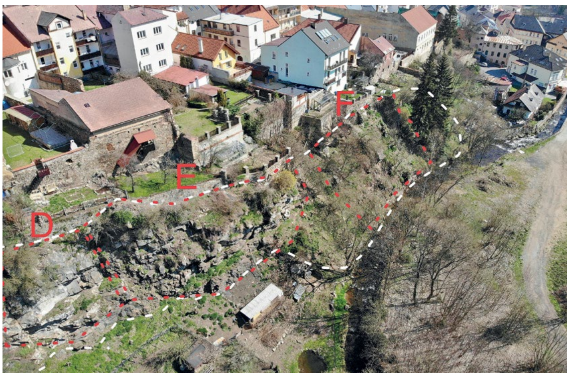
▲ Drone photo of a rock slope in Vimperk, with a white dashed line outlining an area of potential rock fall. Sections D and E marked in red threaten a garden community, the accumulation area for section F is the Volyňka riverbed. Photo by M. Dostálík.
