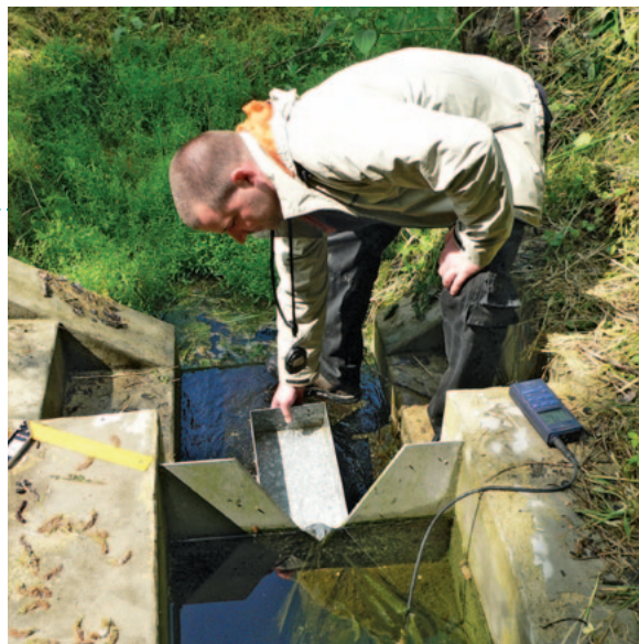
Field measurement and sampling of groundwater from a spring at Radvňovice being carried out for the project Review of Groundwater Resources (author: Z. Novotný).
