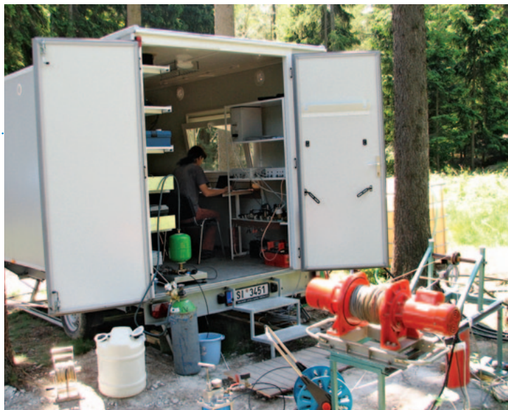
Field measurement of the hydraulic properties of rocks in a borehole at Tis near Blatno being carried out as part of project MIT FR-T11/367 (author: O. Myška).
