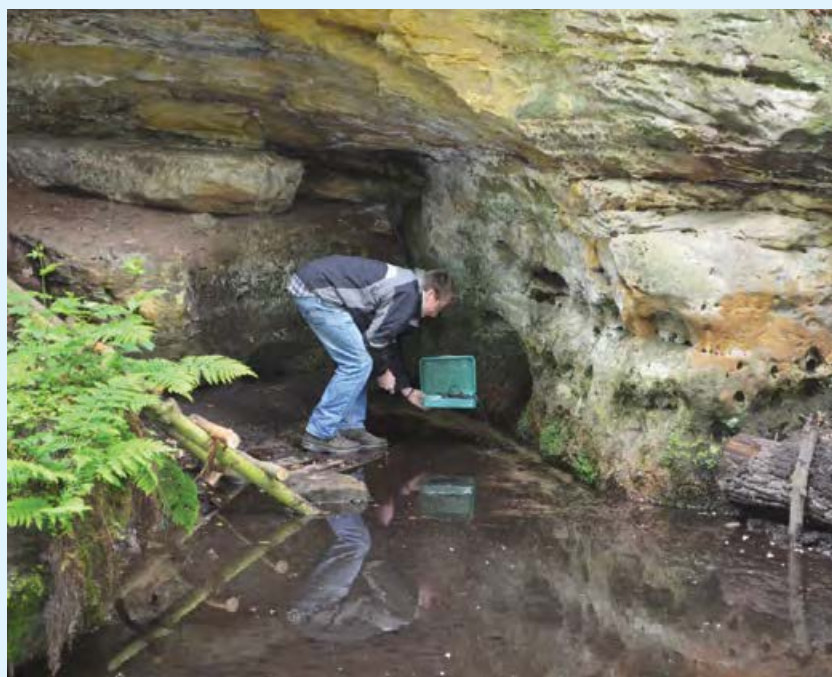
Measurement of the conductivity and temperature of water in a spring emerging from open fissures in sandstones of the Bohemian Cretaceous Basin (photo by P. Fiferina).
