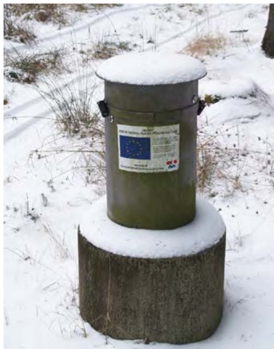
Drill hole to investigate the B aquifer in the Ústí nad Orlicí syncline near Mikuleč.
