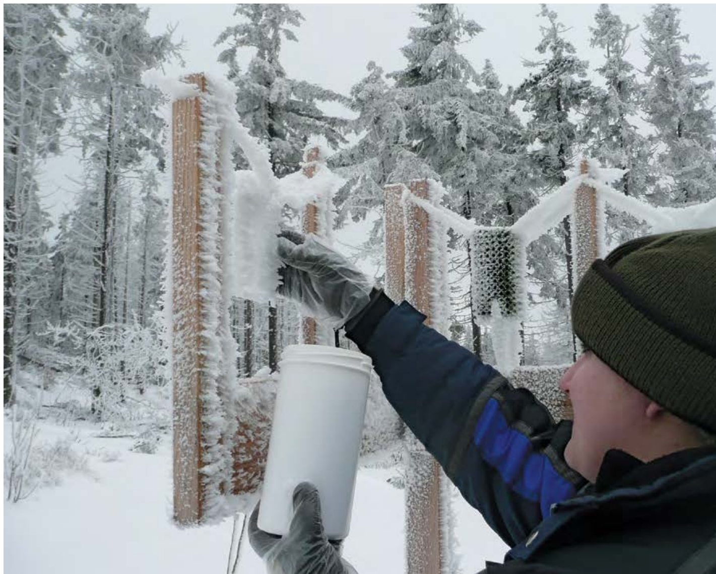
Sampling of horizontal atmospheric precipitation (rime) at the Velký Polom site in the Moravskoslezské Beskydy Mts (photo by K. Hrdličková).
