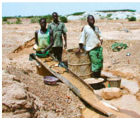
Extraction of gold using a primitive sluice, northern Burkina Faso, 2004
