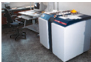
Trace elements in solid materials are measured by the wave dispersed X-ray spectrometer 9400 Advant XP (ARL)
