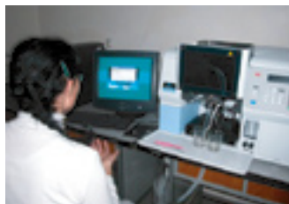
The Perkin-Elmer AAnalyst 100 flame AA spectrometer analyses cations in waters and solid samples
