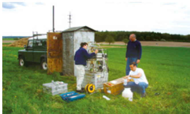
Sampling of subsurface waters from the Cenomanian rocks for radiometric dating, in cooperation with the University of Bern as a part of the BASELINE EU Project
