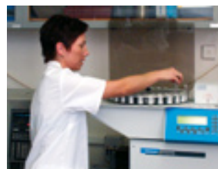
Gas chromatograph with autosampler Tekmar, enables the quick determination of volatile compounds in water and solid samples
