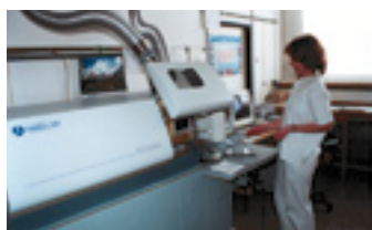
IRIS Advantage Thermo Jarell Ash emission spectrometer: main and trace elements in waters, REE in solid samples
