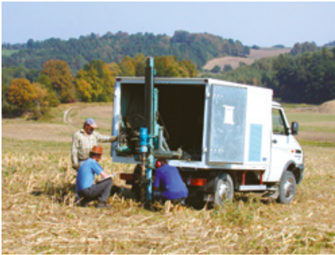
CGS drilling machine LUMESA 353 near Žulová
