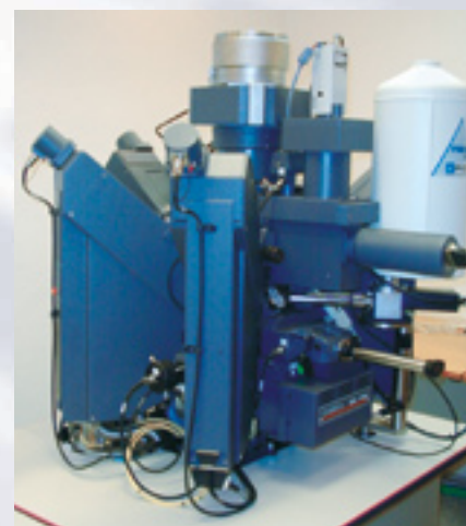
The CAMECA SX-100 electron microprobe, at the joint laboratory of Masaryk University, Brno & the CGS, allows the detection and quantification of elements from B to U, acquisition of SE & BSE images, and the collection of X-ray distribution maps
