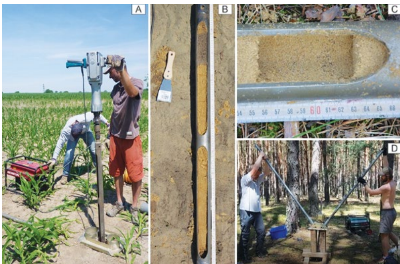
Hand drilling of aeolian sediments in the Moravian Sahara region to distinguish generations of aeolian sediments and sampling for optical luminescence dating. Photo by D. Nývlt.
