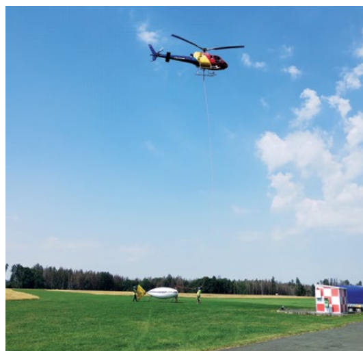
SEMACRET project, airborne geophysics: the FTMG detector is used to search for mineralized structures. Photo by V. Wertich.
