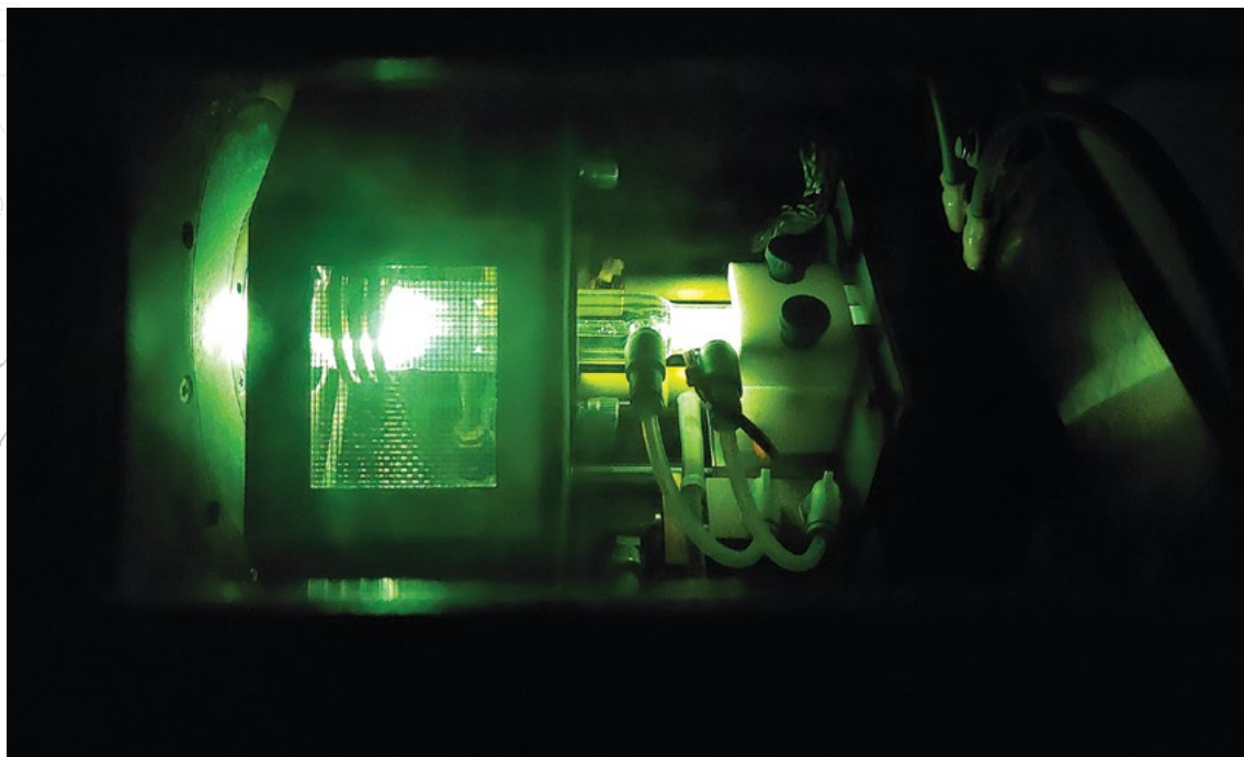
Plasma in Thermo Scientific Neptune mass spectrometer (MC ICP MS). Photo by F. Laufek.
