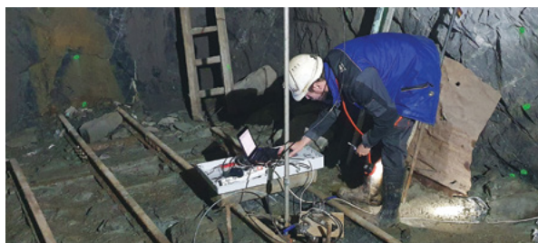
► Water pressure tests in the Bukov II Underground Research Facility in the Rožná mine. Photo by J. Holeček.
