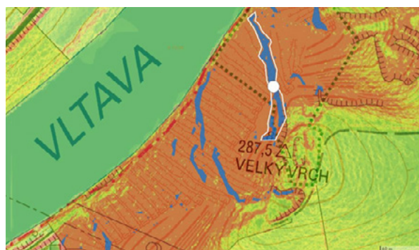
► A white polygon depicts the general slope of a rockfall area in the Větrušická rokle National Nature Reserve on a 5 th generation digital relief model (© ČÚZK). Blue areas mark parts of the terrain with slopes of 50–90°, representing other potential rockfall occurrences.
