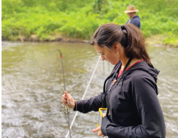
► Measuring the Rokytná River's flow rate with a velocimeter, PERUN project. Photo by R. Hadacz.
