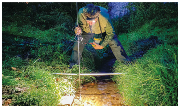
► Measurement of the Oslava River's flow rate with a velocimeter. Photo by R. Hadacz.
