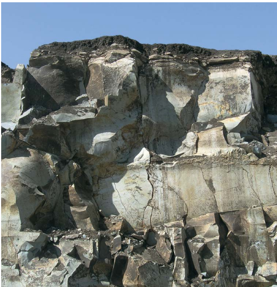
■ View of an outcrop of solid ignimbrite in the wall of the Debre Birham quarry. This rock is abundant in the Ethiopian Highlands and is extracted from numerous small and larger quarries. The material is transported and used for construction and repair of roads and other communications. The aggregate is also used for construction of rockfill dams, many of which are being built at different localities to capture the water falling during torrential rains. Photo by J. Krupička.
