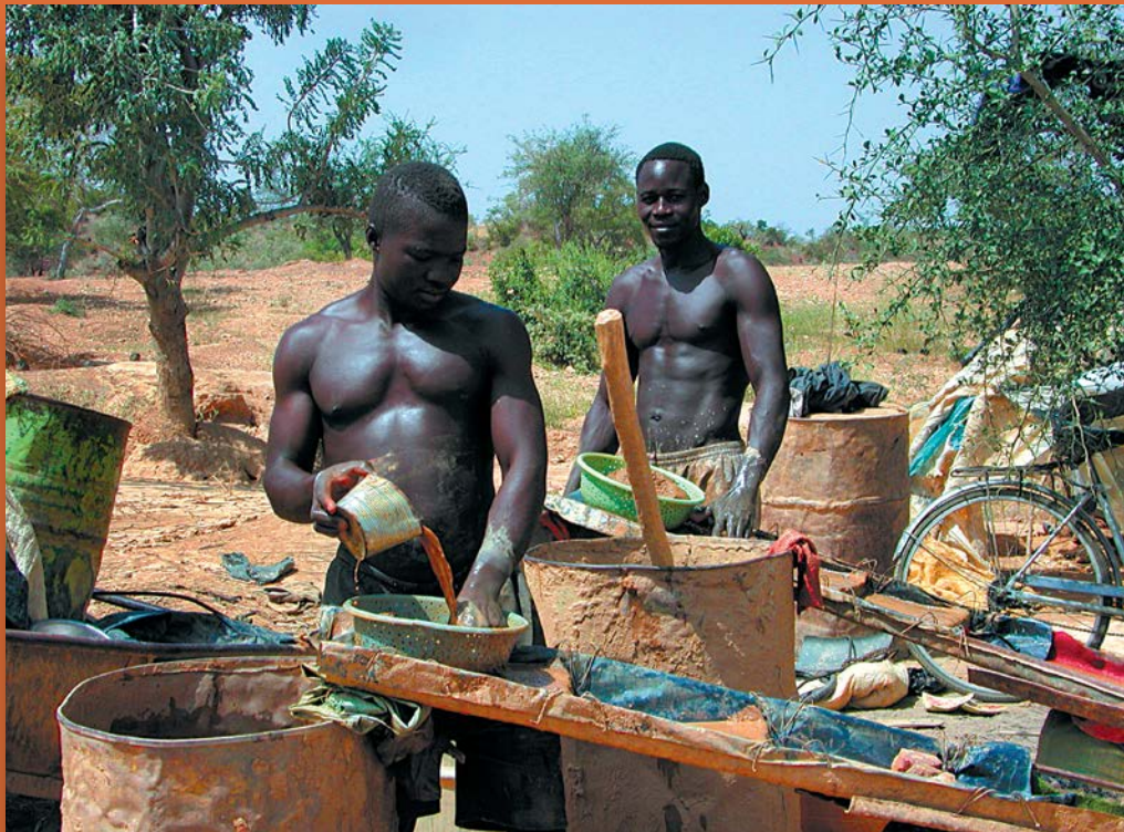
Crushed ore is washed in primitive sluice boxes. Defects in the sluice boxes such as the wrong inclination and irregular water flow, etc. result in poor recovery of gold during gravitational separation. The photograph shows gravitational procedures used for the recovery of gold at Pousghin. Photo by J. Pašava.
