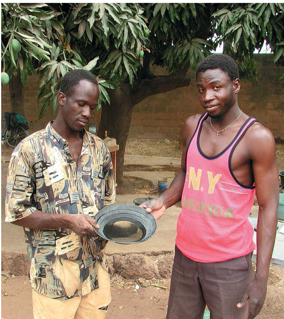
■ Gold concentrate obtained from tailings at the Boutouonou 3 mining operation in eastern Burkina Faso using gravitational methods. Photo by J. Pašava.
