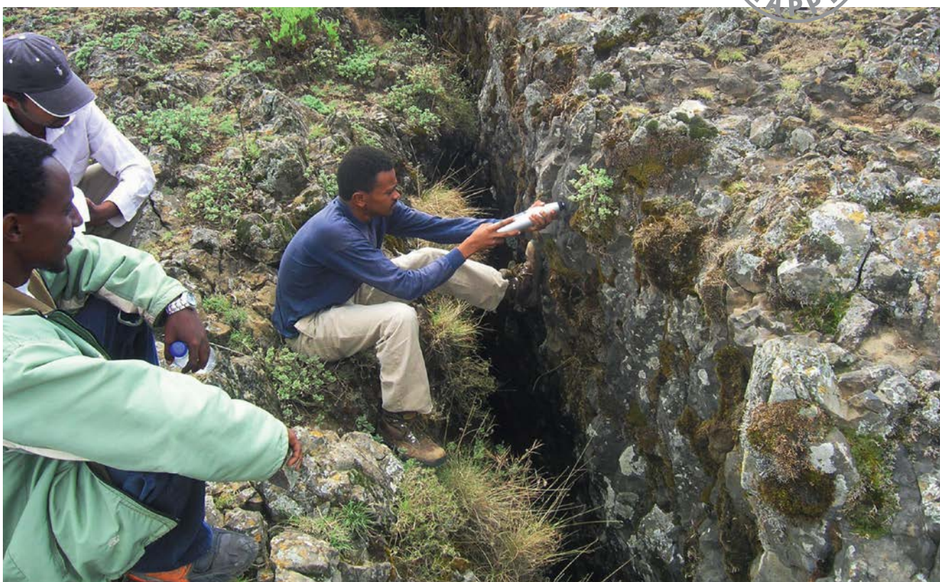
■ A block of basalt at the edge of the River Jemma basin has been loosened. Leta, a geologist from the Ethiopian Geological Survey assisted by his two colleagues Janymar and Eshatu, is testing the basalt block using a Schmidt or Swiss hammer to measure the elastic modulus of the rock. Photo by J. Krupička.
