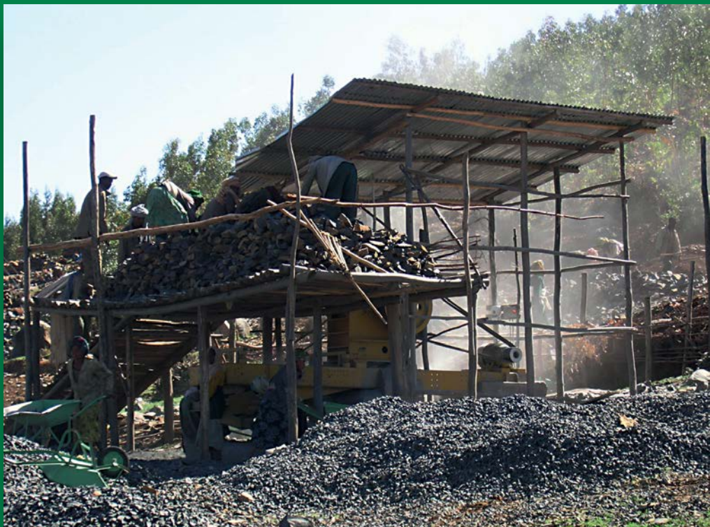
A quarry for extraction of ignimbrite lies close to the town of Debre Birham. The rock is used to construct and reinforce roads in Ethiopia. Work is predominantly manual and women are often employed in crushing the rock for the production of aggregate. Photo by J. Krupička.
